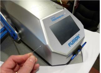
4) Remove the display enclosure by prying it free from the bottom and pulling the entire enclosure up from the press. See Figure 5
