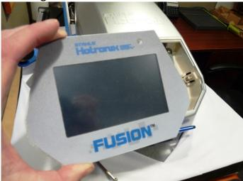
5) Turn the display enclosure over. There will be a MicroSD card on the bottom-center of the unit's motherboard. See Figure 6
