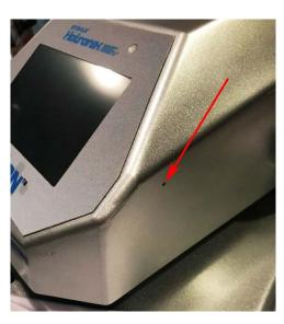
3) Use a paperclip or similar tool to release the clasps holding the display enclosure in place. Use a small screwdriver to prop up the released side while releasing the opposite side. See Figures 3 & 4
